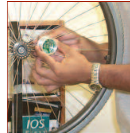
Approximately the size of a roll of 35-mm film, the Data Logger can precisely measure wheelchair velocity, time of day, and distance traveled over a period of weeks. The Data Logger was developed and tested at UPMC-SCI.
