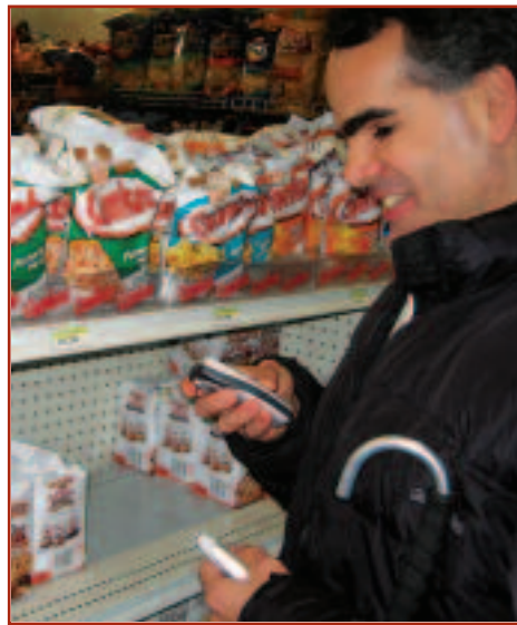
Dan Rossi, who has been blind from early childhood, uses "Trinetra" to identify items on the grocery store shelf. Trinetra is not a new technology, but an innovative combination of existing technologies. A UPC-reading pen uses the operator's cell phone to send codes over the Internet to the UPC database; the information sent back to the phone uses software that translates the signal into electronic speech.
